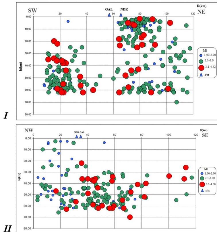
*Fig. 3. Seismological cross-section of earthquakes with  $m_l \geq 1.0$  of the Absheron zone on the I-I and II-II profiles in 2003–2023*
