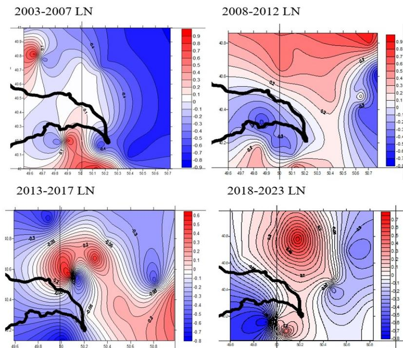
Fig. 5. Distribution map of the Lode–Nadai coefficient as a result of the orientation of compression and tension axes of earthquake source mechanism  $m \geq 3.0$  in the Absheron territory during 2003–2023.
